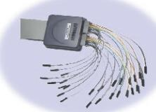
AT-LA500 provides a dedicated expansion bus, called AT-XSS, for expandability and synchronization with external instruments (i.e. oscilloscopes).
