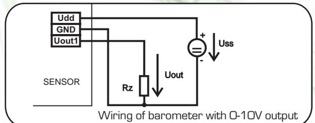
Wiring of barometer with 0-10V output
