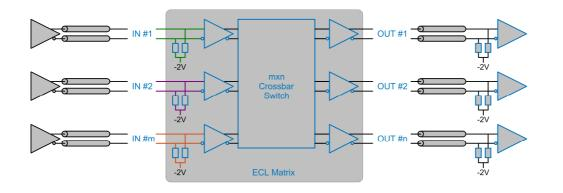
The KSD0490 is capable of switching data rates up to at least 650 Mbit. The system supports come with serial and Ethernet control interfaces, allowing setup flexibility and easy remote test management.
