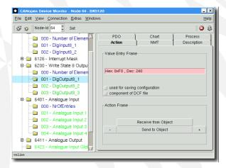
The information on how to display the device object dictionary is obtained from the EDS file of the device (EDS - Electronic Data Sheet, text- or XML format according to ISO 15745) or can be scanned from the device directly. Special device configurations can be loaded, stored and scanned from DCF files. Additionally, configurations of complete networks can be saved in project files.
