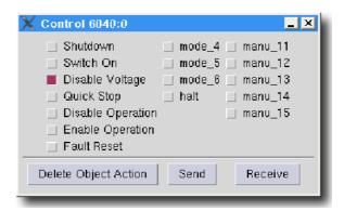
Values of manually configured device objects can be stored to a file and reloaded into the device.
