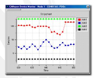
The integrated process image summarizes the most important process variables of the network. The data can be received via SDO and PDO. The PDO tab allows the simple configuration of the PDO-Mapping by Drag&Drop. Additionally PDOs can be sent and received and data from received PDOs can be plotted in a stripchart with one click.
